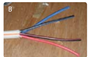
Two conductor wire (A) is used when running wire directly to a speaker, while 4-conductor wire (B) is often used for runs to volume controls.
