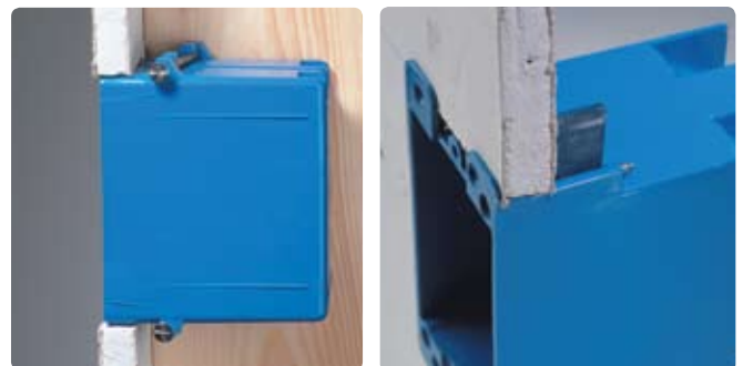
A junction box or "J-box" provides a clean-looking and safe interface for your in-wall speaker cable to exit your wall and run to your receiver. J-boxes made for retrofit installation have rotating tabs that secure them to your drywall. If you're installing a J-box to run speaker wires to your receiver, mount it at the same height as AC outlets for a clean, uniform look. If you're installing one for an IR sensor or volume control, mount it at the same height as light switches.
