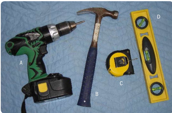
Some of the tools you'll need to pre-wire your home include: (A) a power drill; (B) a hammer; (C) measuring tape; and (D) a level.
