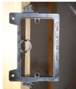
Backless brackets provide the minimum structure you'll need to attach a wall plate. If you're installing one to run speaker wires to your receiver, mount it at the same height as AC outlets for a clean, uniform look. If you're installing one for an IR sensor or volume control, mount it at the same height as light switches.
