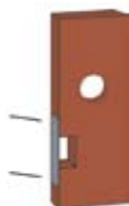
Use nail plates if you notch studs or joists, to prevent your speaker cable from being damaged in the future.
