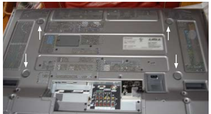
Like most flat-panel TVs, the one pictured above has four plastic caps over the holes used for wall-mounting. You can use a screwdriver to pry them off.
