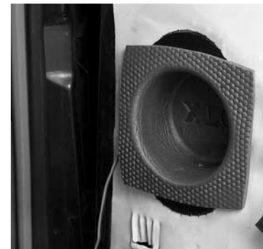
Speaker baffles help minimize damage to a speaker resulting from dust or moisture.
