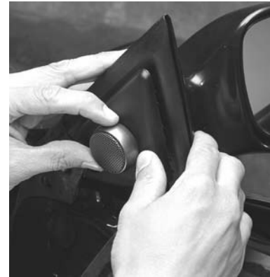
A surface-mount tweeter (shown here in door sail panel) is an easy way to improve your system's sound.
