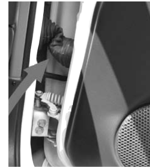
The rubber boot that protects your door wires' journey to the dash is a great place to house your speaker wires.
