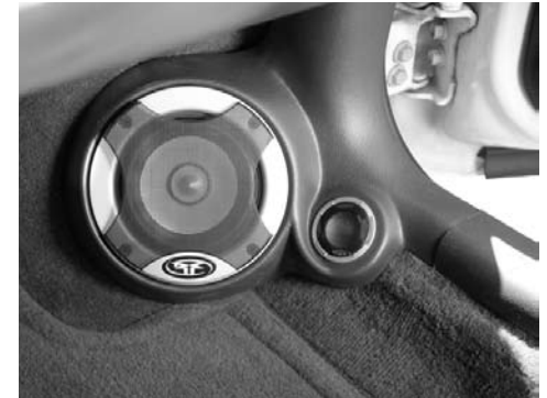
Install your woofer in your door or in your kick panel (shown above right in a Q-Logic kick panel pod).
