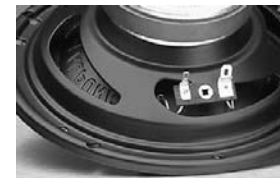
Be consistent with how you attach wires to your speaker terminals, to avoid phase distortions.
