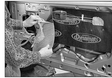
Use speaker baffles or a Dynamat kit to reduce extraneous noise.
