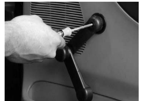
As the first step of removing the door panel, unclip or unscrew the window crank.
