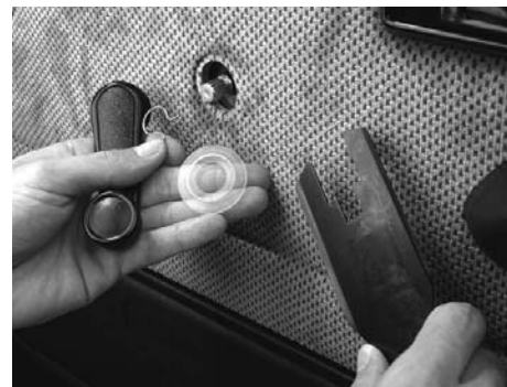
As the first step of removing the door panel, unclip or unscrew the window crank.
