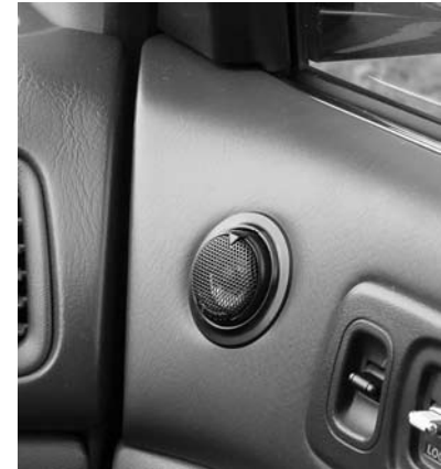
Install your woofer in your door or in your kick panel (shown above right in a Q-Logic kick panel pod).
