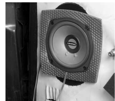
Speaker baffles help minimize damage to a speaker resulting from dust or moisture.
