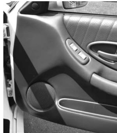
Install your woofer in your door or in your kick panel (shown above right in a Q-Logic kick panel pod).
